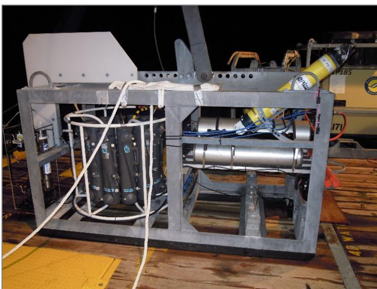
Figure 1. Towed platform used for mapping plume extents of the Deepwater Horizon oil-spill shown with a sensor suite (UMS included) and Niskin Samplers.
